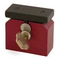
Test all keys to make sure the cylinder is keyed correctly.
