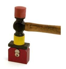
Use a plastic, rubber or rawhide mallet to set the brass strip. The use of a steel hammer is not recommended as repeated use will damage the top plate.
