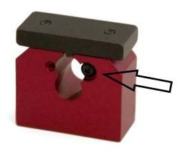
The CCT-100 block is adjustable for both 6 and 7 pin cylinders. With the stop screw in the counter bore, 6 pin cylinders can be accommodated. Move the stop screw to the other side for 7 pin.
