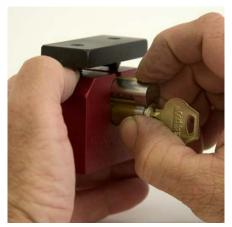
Lift the spring loaded top plate and slide the cylinder into the capping block. The spring tension will hold the brass strip in place.
