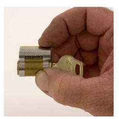
After keying the cylinder, place the brass cover strip on top of the cylinder and hold in place.
