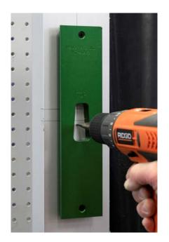
Drill a 3/8" or larger starting hole for the router bit in the center of the template hole to be routed. In the picture we are using a step drill bit.
