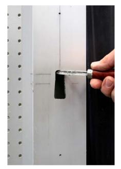
Clean the area of left over cutting lube and chips. Use a machinist scraper or an aluminum cutting file and deburr all of the openings.
