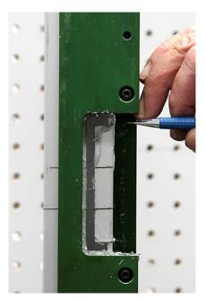
Note that we did not route through the top of the lip area, this will be cut out with the next pass. If you run through the side wall you run the risk of hitting the template with the router bit.
