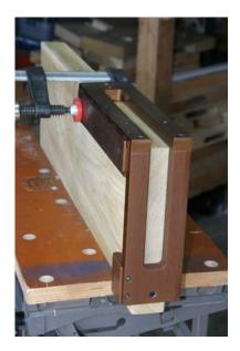
A c-clamp may be used to secure the template as shown.
