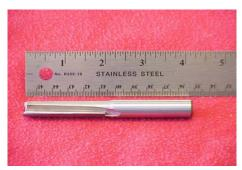
Choose a router bit long enough to reach the bottom of a flush bolt mortise. The router must also have enough throw to reach.
