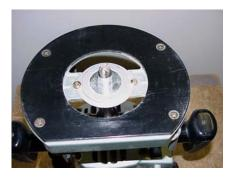
Router base with 5/8" template guide and 1/2" router bit
