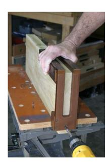
Secure template to door. This is accomplished with the use of a dry wall screw in the top and front of door. The hole left on the top of the door will not be seen. The hole on the front of the door can be patched with a dab of putty, or a finish screw can be installed and it will look like part of the installation. See next picture for an alternate method of attaching.
