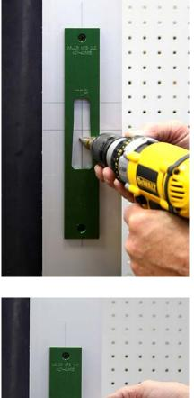
Drill a 3/8" or larger starting hole for the router bit in the center of the template hole to be routed. In the picture we are using a step drill bit.
