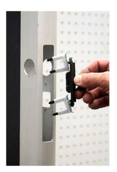
Our LMB-08 mounting brackets and LMB-089 tool are being used to mount the lock in the channel. The door can also be drilled and tapped for lock mounting tabs. We do not advise drilling and tapping the rear of the channel like factory doors. They are drilled and tapped prior to the glass being installed, you will be drilling and tapping into a glass channel. **You run a great risk of breaking the glass in the door!**
