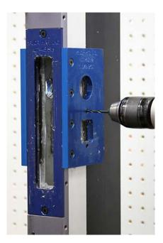
Drill the mounting holes for the indicator with a #21 drill bit.
