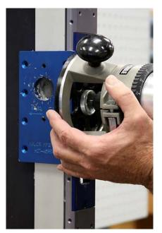
Route the faceplate opening last. When completed, again brush away the chips and make a second pass. We recommend making this cut last because of the unlikely event of a broken router bit, the large faceplate hole will be covered by the router base and the broken bit will most likely be contained in the channel.
