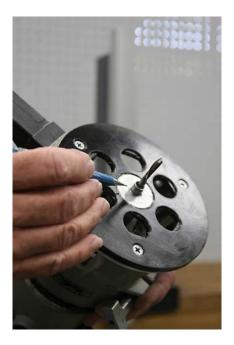
Your router needs to be equipped with a 3/8" outside diameter template guide mounted in its base. *Failure to use a template guide will cause the opening being routed to be too large and may damage your HIT-45 templates or the door.*
