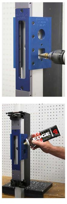
Here we are drilling the starter hole for the lock indicator. If you are not using an indicator in your installation, do not drill this hole.
