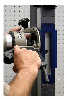
Use the same procedure and route the opposite side of the door. Don't forget to brush out the chips and make a second clean up pass.
