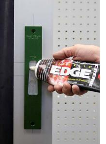
We recommend the area to be routed be lubricated with a cutting lube. We use a product called Tapmatic Edge Cream made by the LPS Company. You can find this product at industrial hardware stores or machine shop supplies. This is also a handy product to use for other drilling or tapping chores.
