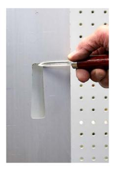
Clean the left over cutting lube and chips from the frame. Use a machinist scraper or an aluminum cutting file and deburr all of the opening.
