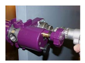
The draw die is placed inside door with the "ears" toward the folded side of the door. The opposite side of the door has a seam that is welded.
