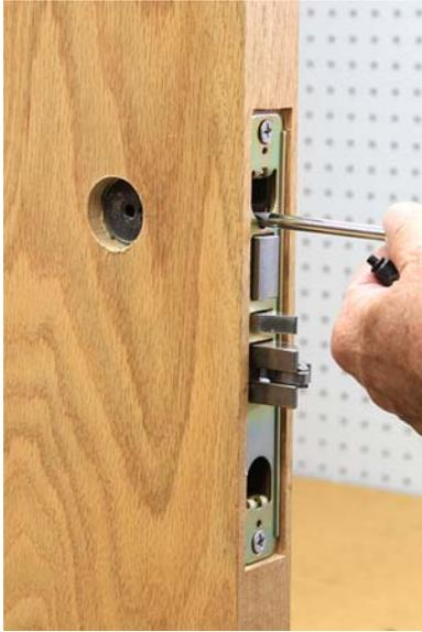
The cylinder hole is large enough to remove the HIT-22 without having to remove the mortise lock from the door. Simply screw the extractor handle into the HIT-22 guide, loosen the mortise cylinder retaining screw and the HIT-22 can be removed.
