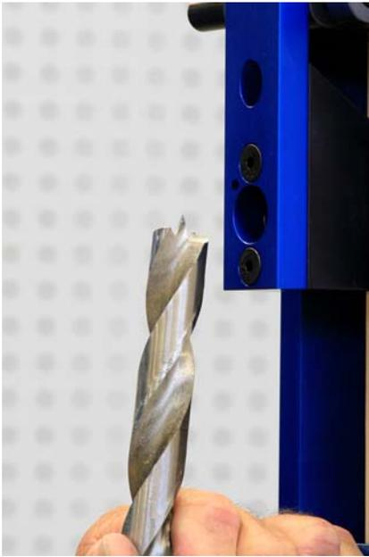
Use a 3/4" brad point bit to drill the hole for the door position switch. Use this bit on wood doors only.
