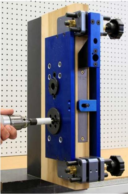
Using a good quality hole saw, drill the spindle hole using the drill bushing shown in the picture. The hole saw size is 3/4" and is drilled to the mortise pocket on both sides of the door. Use a slow speed when drilling.
