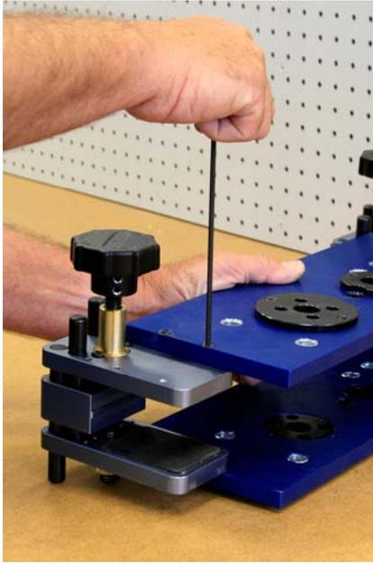
With both clamps opened equally, install both inside and outside templates to the HIT-66 clamp as shown. Do not tighten the 10-32 screws at this time. When all screws have been loosely installed, then it is ok to tighten.
