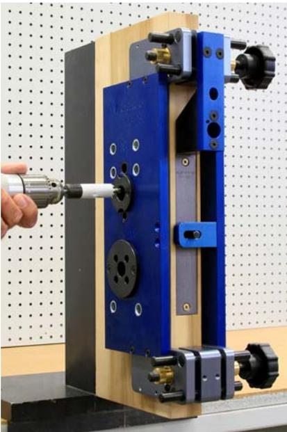
With the 3/4" hole saw still in the drill, drill the 3/4" wire run hole. Drill half way from both sides of the door. Use a slow speed when drilling.
