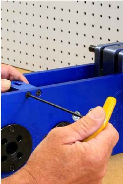
Install the alignment guide to either side of the template set. This is used to align the template with the mortise pocket.
