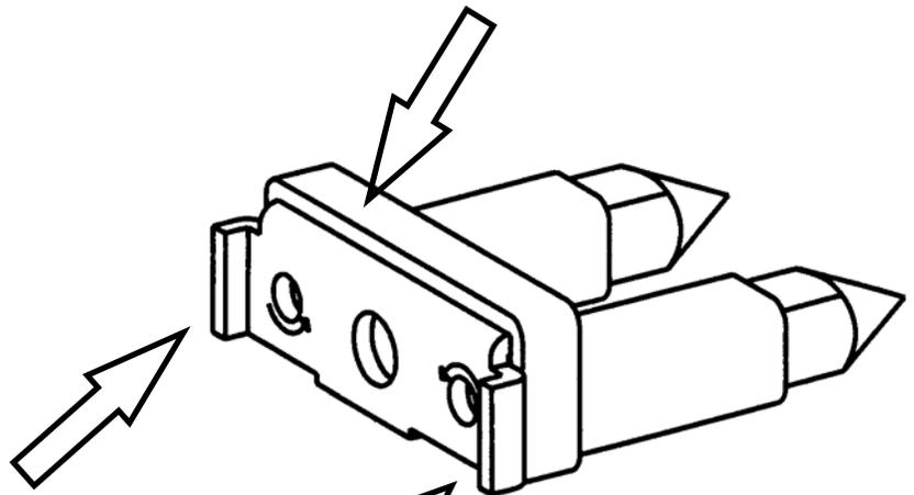
The plastic adapters shown at the right will snap on the ears of the LMB-08 mounting bracket and adapt it to different door types. To mount the adapters properly, make sure that the number on the top of the adapter is right side up when facing the plastic strip on the mounting bracket.
