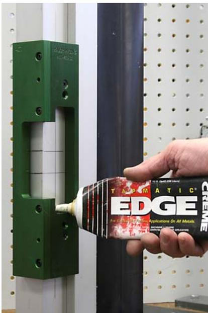
Template mounted and ready to go. We recommend the area to be routed be lubricated with a cutting lube. We use a product called Tapmatic Edge Cream made by the LPS Company. You can find this product at industrial hardware stores or machine shop supplies. This is also a handy product to use for other drilling or tapping chores.
