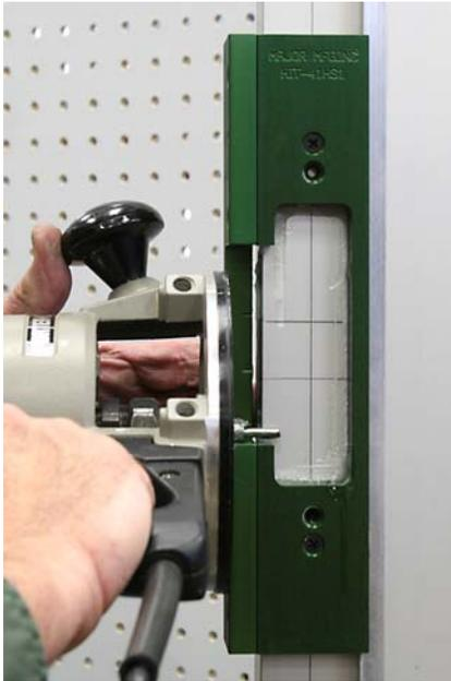
Adjust the router bit so it is about 1/4" past the aluminum as shown.
