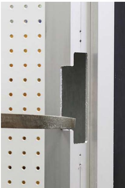
Don't forget to square off the corners for the lip area in front of the front of the frame, the router will leave these round.
