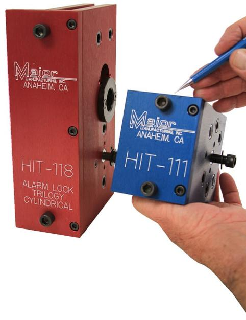
This drill guide is now equipped with an adjustable backset. With the backset studs outside as shown, it is a 2-3/4" backset. With the studs moved to the inside of the plate, it will center on a 2-3/8" backset on a 1-3/4" door. Make sure studs are threaded in snug.
