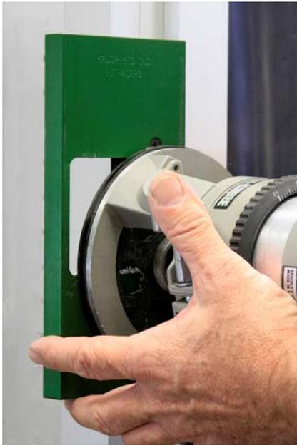
Place the router bit in the starting hole and with firm control of the router follow the HIT-40 template and feed the router slowly in a **CLOCKWISE DIRECTION**.
