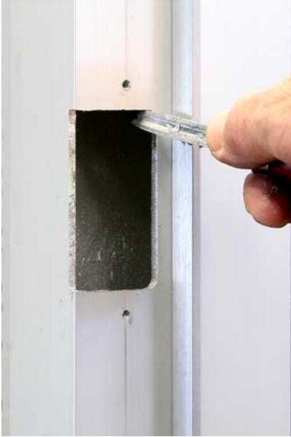
Remove the router template , clean off the lube and de-burr the sharp edges with scraper or file.
