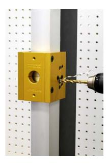
Change to a 1/4" bit and drill the hole for the rim cylinder tailpiece.
