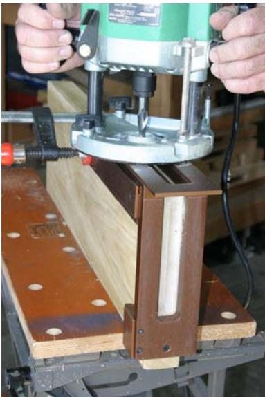
**DO NOT ATTEMPT TO MAKE THIS CUT IN ONE PASS!! ROUTE NO MORE THAN 1/4" AT A TIME UNTIL PROPER DEPTH IS REACHED.**
