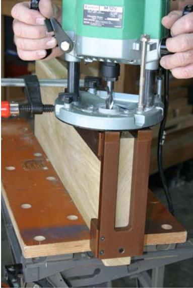
Adjust the depth of cut on the router and route the faceplate cut out. After routing the door face, route the top of the door.
