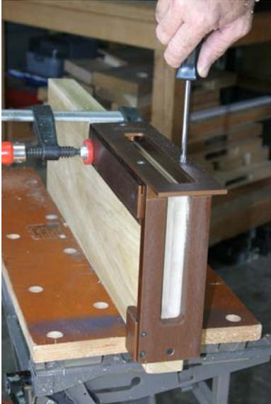
Attach the template for the mortise cavity, re-adjust the router depth and route the mortise cavity.
