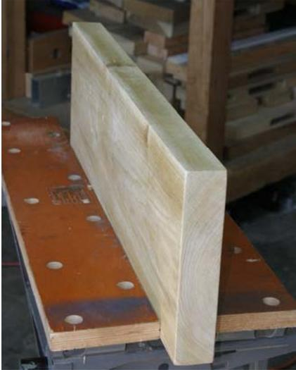
For flush bolt installation, door must be removed from jamb. Secure in a door stand for ease of installation.
