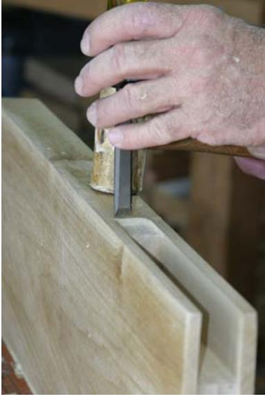
After routing the opening, square the corners with a chisel. This can be accomplished with a standard wood chisel or with the use of a corner squaring chisel.
