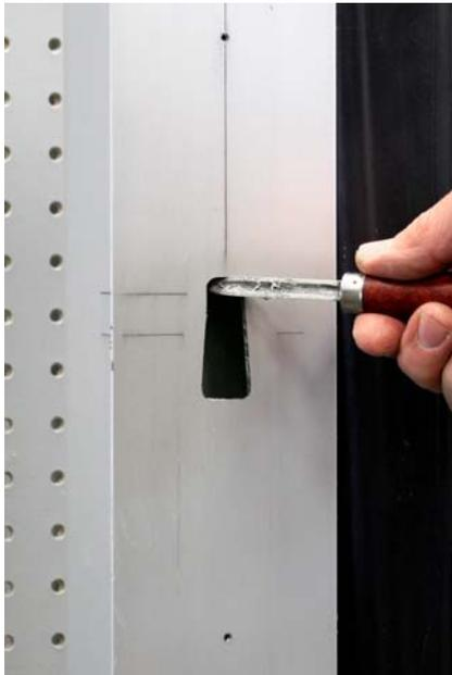
Clean the area of left over cutting lube and chips. Use a machinist scraper or an aluminum cutting file and deburr all of the openings.
