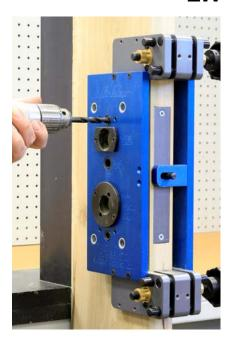
To install Sargent LW Trim, use a 3/8" drill bit and drill the two holes marked LW on the drill guide. Drill half way from both sides of the door. Back the drill bit when drilling to clear chips from the drill bit.
