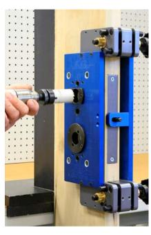
Start by drilling the mortise cylinder hole. Use a 1-1/4" hole saw and drill only on the side of door that the cylinder will be on.
