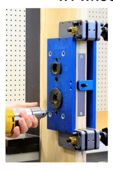
To install Sargent WT Trim, use a 1/8" drill bit and drill the for holes marked WT on the drill guide. These are pilot holes for mounting screws, drill to a depth of the screw length.
