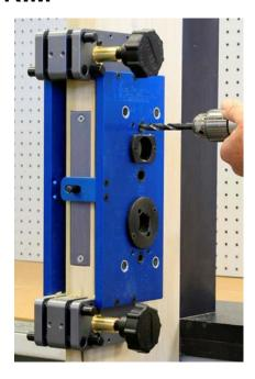
Remove HIT-66 drill fixture from door and install lock and trim per manufacturers directions.
