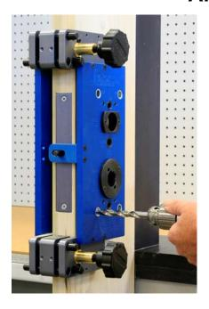
To install Sargent Anti-Vandal Trim, use a 7/16" drill bit and drill the four holes marked AV on the drill guide. Drill half way from both sides of the door. Back the drill bit when drilling to clear chips from the drill bit.
