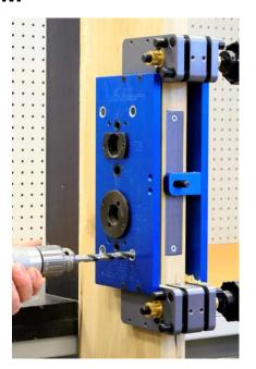
Remove HIT-66 drill fixture from door and install lock and trim per manufacturers directions.
