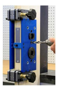
If your mortise lock requires a thumb turn inside, use a 1/2" diameter drill and drill to the mortise pocket. Drill the inside of the door only.
