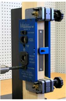
Drill the escutcheon holes half way from both sides of the door. When all holes have been completed, remove the HIT-66 drill guide from the door.
