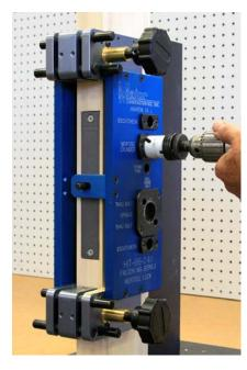
Use a 1-1/4" hole saw to drill the mortise cylinder hole on the outside of the door. When all holes have been drilled, remove the HIT-66 drill guide from the door. This is a prep for a Falcon MA series mortise lock with rose trim. If installing escutcheon trim see next page.
