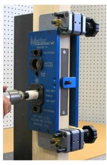
Using a 1-1/8" hole saw, drill the hole for the lock spindle. It is drilled to the mortise cavity.
