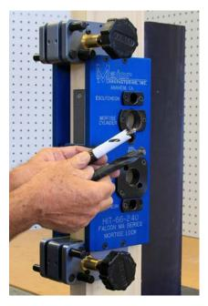
If installing escutcheon trim, the holes can be drilled with a twist drill or hole saw. The factory template calls for a 19/32" hole. Our drill guide uses a template hole size of 5/8".
