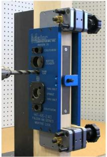
If your mortise lock installation required an inside thumb turn, use a 1/2" twist drill and drill the required hole on the inside of the door only.
