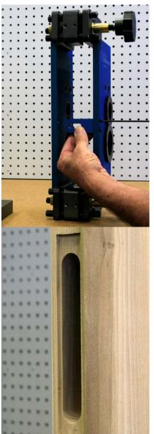
Install the alignment guide to either side of the template set. This is used to align the template with the mortise pocket.
