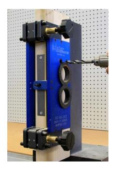
Using a 1/2" twist drill, drill the two upper holes. Drill these half way from both sides of the door.
