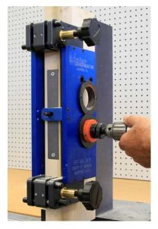
With a good quality hole saw, drill the two 2-1/8" holes to the mortise pocket.
