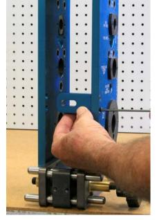
Install the alignment guide to either side of the template set. This is used to align the template with the mortise pocket.
