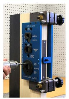
Start by drilling all of the required 3/8" diameter holes used for the thru bolts. We are drilling the lower holes above and below the mortise lock spindle hole. These holes go to the mortise pocket. Use a standard twist drill for wood or metal doors.
