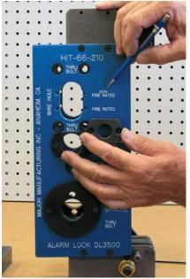
There are two positions for the wire hole. One for fire rated doors and the other for non-fire rated. Choose the location and install the 3/4" diameter drill guide.
