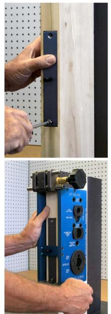
Install the mortise lock positioning plate. The plate will fit into the 1-1/4" x 8" faceplate cut out. There will be a 3/8" diameter pin centered on the plate. There is no top or bottom to worry about.
