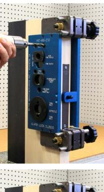
Drop down and drill the last two thru bolt holes. They are drilled to the mortise pocket on both sides of the door.
