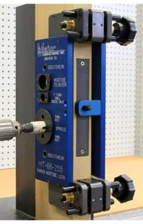
Change to a 1" hole saw and drill the spindle hole. Use a slow speed and back the hole saw out a few times to clear the hole saw from chips. Drill to the mortise pocket from both sides of door.
