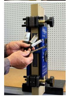
For this installation you will need 5/8", 1" and 1-1/4" hole saw. Also required will be a 3/8" diameter twist drill.
