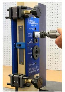
The mortise cylinder hole is drilled next with a 1-1/4" hole saw. Drill only on the side od the door that requires a cylinder.
