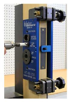
The last hole to be drilled is for the thumb turn if required. The factory template calls for either a 5/8" or 7/8" hole depending on rose or escutcheon trim. A 5/8" works for all the escutcheon trim tested. Drill on the inside of door to the mortise pocket.
