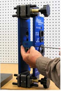
Install the alignment guide to either side of the template set. This is used to align the template to the mortise pocket.
