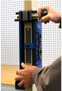
Slide the HIT-66 alignment fixture over the alignment pin and tighten to door. Alternate tightening between the top and bottom clamp. Do not attempt to tighten one clamp all the way at once.
