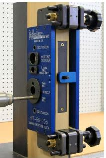
Opposite side of thru bolt holes being drilled.
