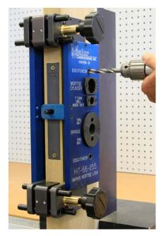
If the lock being installed requires thru bolt holes for escutcheon trim, drill them now with the 3/8" bit still in the drill. Drill half way from both sides of door, top and bottom.
