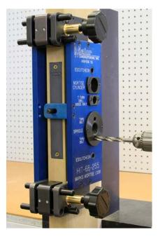
Start by drilling the thru bolt holed located above and below the spindle with the 3/8" diameter drill bit. Drill both sides of door to the mortise pocket.
