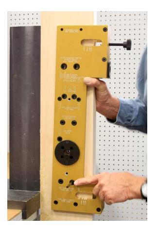
Slide the pin thru the corresponding drill guide hole and into the door. The pin does not need to go thru to the bushing on the other side.
