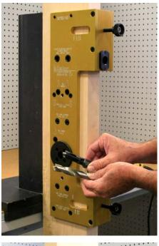
The drill guides on this jig will accept both twist drills and hole saws. For this wood door install we are using a brad point twist drill.
