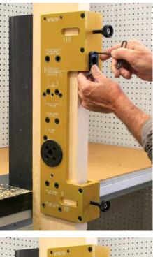
The drill bushing for the DPS on the edge of the door is adjustable for centering on a 1-3/4" door.
