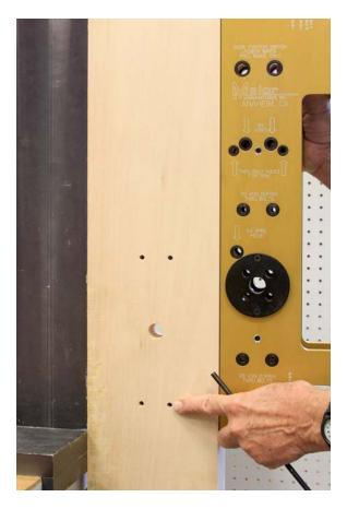
Choose any one of the four corner thru bolt holes and align with the supplied pin. Here we chose the lower RH hole.
