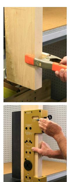
To help support the weight of this template, use a spring or "C" clamp as shown.
