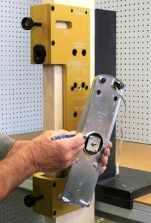
The two screws around the spindle on the outside trim will require a small relief so the trim will be flat on the door. Use a 3/8" drill bit and drill to a depth of about 1/4". This hole does not need to go to the mortise pocket, just dimpled.
