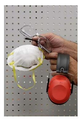
These are the most important tools that you will use in this installation. Always use eye and ear protection when routing wood doors and jambs.
