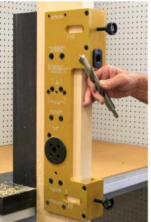
The DPS requires a 3/4" diameter hole. If drilling on a wood door use a brad point drill bit as shown. If installing on a steel door, use the 5/16" drill bushing adapter and twist drill. After the HIT-32-380 has been removed from the door, enlarge to 3/4" with the use of a step drill. **DO NOT USE A HOLE SAW FOR THIS STEP, THE FINISHED HOLE WILL BE TOO BIG!!**
