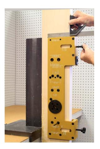
With the pin in the door, the backset and height are now set, Just use the two black knobs to square the device
