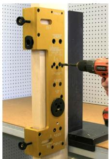
A second RX hole is needed as shown. Match this hole with the trim for the hand of the door. Drill with a 3/8" bit half way from both sides of the door.
