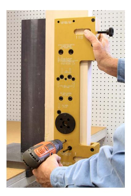
Attach to door on the inside using two drywall screws. Use the directions starting on page 5 to install.
