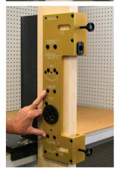
There are 4 thru bolt holes for the 99 device, drill these holes with a 1/4" diameter drill bit half way from each side of the door.
