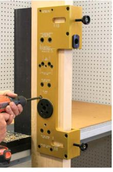
Drill the RX hole as shown with a 3/8" drill bit half way from both sides of the door. Note: The factory template shows a 13/32" Hole but a 3/8" works fine.
