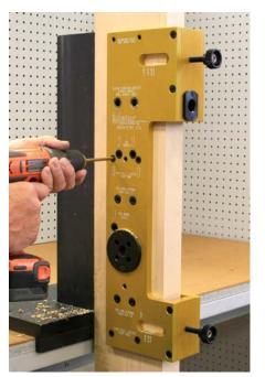
There are four drill guide bushings marked 99 Von Duprin thru bolts. Two at the bottom of the drill guide and two about 1/3 of the way down. Drill all four with a 1/4" drill bit half way from both sides of the door.
