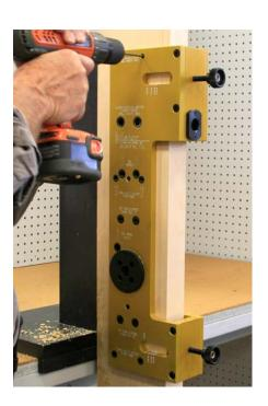
The last holes needed are for the control box located on the interior of the door. Drill two 5/32" holes to a depth of 1" on the inside of the door only.
