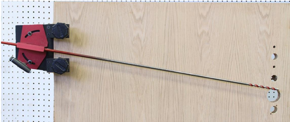
The full length drill bit inserted in the drill guide. By having the 3/8" rod and drill bit inserted at the same time, you can see where the drill bit will make contact to the door and where the hole will end up.
