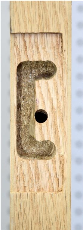
Completed wire raceway hole shown at the right.
