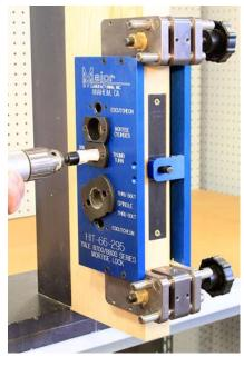
Drill the thumb turn hole with a 3/4" hole saw. Drill to the mortise pocket only on the side of the door that the thumb turn will be on. When drilling pull the hole saw out of the cut several times to clear the chips, use a low rpm.
