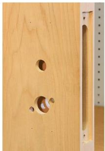
Remove the HIT-66 clamp, template and alignment plate from door.
