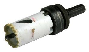
All hole saws are not created equal. A cheap hole saw from a home improvement center or one that has been dropped can be out of round and will not fit the drill bushings in our templates.
