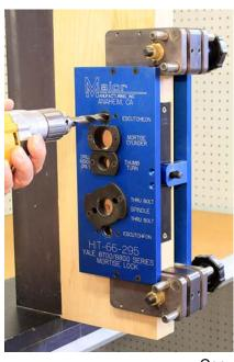
If installing thru bolted trim, use a twist drill and drill the two holes marked escutcheon. Drill half way from both sides of the door.
