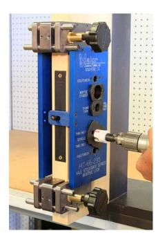
Drill the spindle hole next with a 1-1/8" hole saw. Drill to the mortise pocket on both sides of the door. When drilling pull the hole saw out of the cut several times to clear the chips, use a low rpm.
