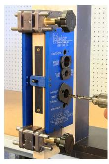
Start by drilling the 5/16" diameter thru bolt holes located around the spindle. A standard twist drill will work on both wood or steel doors. Drill to the mortise pocket from both sides of the door.
