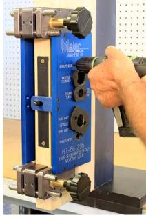
If installing on a wood door, use a 1/16" twist drill and drill the four drill bushings marked escutcheon on both sides of the door. If installing on a steel door, enlarge these holes with a #32 drill bit after removing the HIT-66 from the door.
