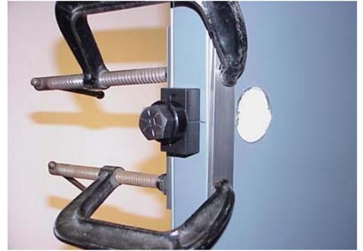
Use an 1-1/8" box end wrench or socket to tighten bolt. This works better than an adjustable wrench. Tighten until the forming die bottoms out on the draw die inside the door.
