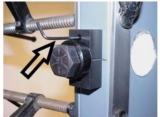
Completed latch face pocket. Drill the two marks left by the set screws with a #29 drill and tap 8-32.
