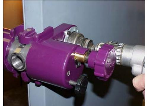
The draw die is placed inside door with the “ears” toward the folded side of the door. The opposite side of the door has a seam that is welded.
