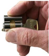
After keying the cylinder, place the cover strip on top of the cylinder and hold in place.
