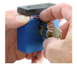
Lift the spring loaded top plate and slide the cylinder into the capping block. The spring tension will hold the brass strip in place.
