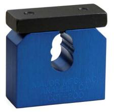
The CCT-200 block is machined to accept the Sargent Removable core from either side, there is no front or back. The core will go in or out with the control sleeve in the locked or unlocked position.
