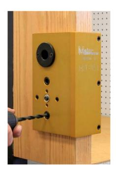
Start by drilling the two post holes. They will require a 5/16" twist drill. Drill the two holes half way from both sides of the door. When drilling, back the drill out several times to help remove chips. Drill both top and bottom holes.
