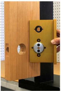
The HIT-151 set consists of both inside and outside drill guides. All required holes are lined with hardened bushings.
