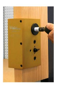
When all holes have been completed, remove the HIT-151 drill guide from the door.
