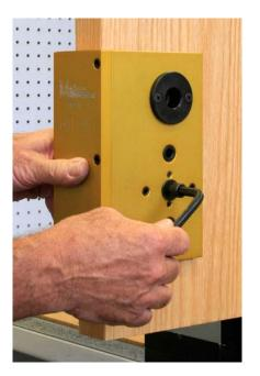
Use the supplied 3/8" socket cap screw to fasten both templates together. Just snug the two plates together.
