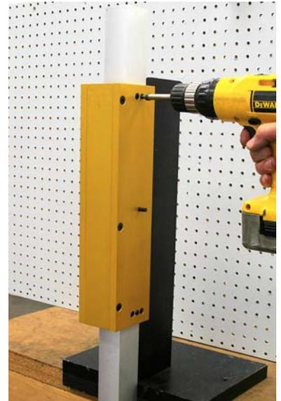
Remove the HIT-22 locating tool. A handle is supplied that makes the job easier.
