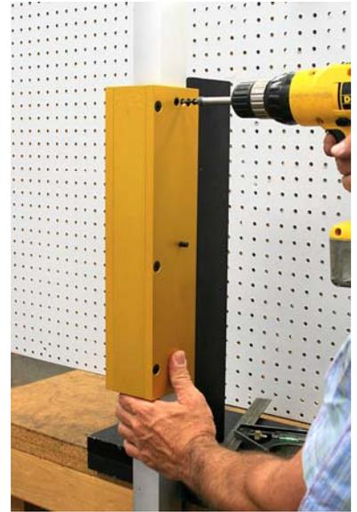
Drill four 7/32" holes on both sides of the door using the drill bushings located at the corners.
