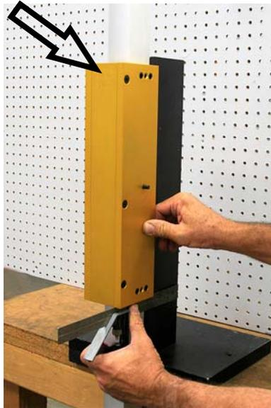
Use the drill screws that were supplied with the guide and attach one using an electric drill. **NOTE:** A drill with a clutch drive is a big help, you do not want to snap a screw in the door. The screw mounting holes are located between the drill bushings top and bottom. Screw only to one side of the door.
