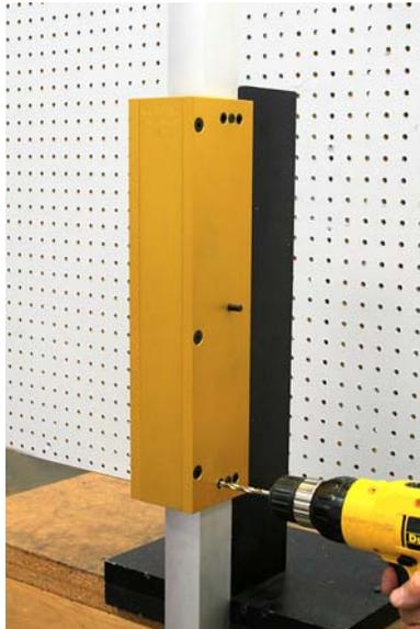
Remove the two drill screws holding the guide to the door.
