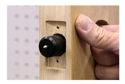
Don't forget to mark the jamb for the strike plate. Shown is our HIT-44SL8 strike locator.
