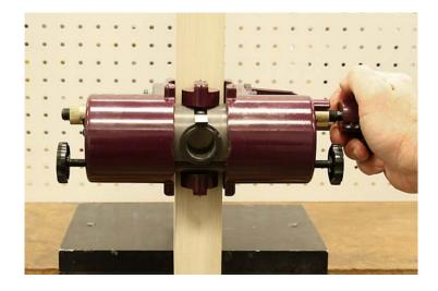
One final turn of the main clamp knob will secure the HIT-44 to the door.
