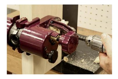
Drill the cross bore first using the proper size multispur bit and corresponding break out plate on the opposite side. USE A LOW RPM WHEN DRILLING AND BACK OUT THE BIT FROM TIME TO TIME TO REMOVE CHIP BUILDUP.
