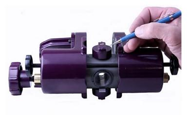
To adjust for 2-3/8" or 2-3/4" backset locks, just rotate the backset knob both on the top and bottom.
