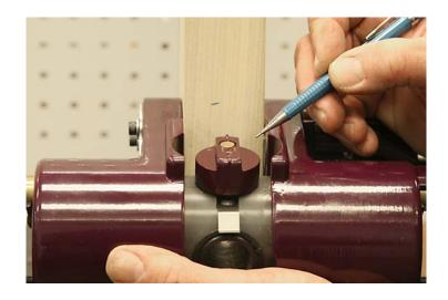
Prior to clamping the HIT-44 to the door, check to make sure the backset adjustment knobs correspond to the lock you are installing. A 180 degree turn of the knob will change the backset to 2-3/8" or 2-3/4"
