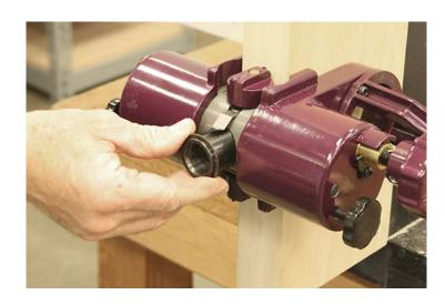
When the cross bore has been completed, drill the edge bore. Snap in the proper size bushing for the job.
