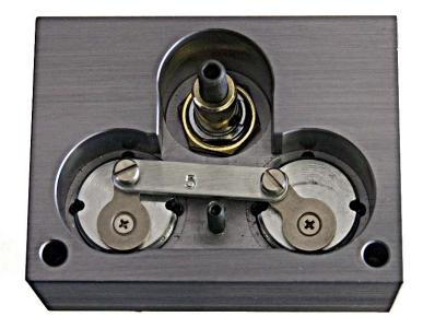
Completed installation of the Schlage Interchangeable core cylinders. Link will allow only one key to be removed at a time. Returning one key will allow removal of the other.
