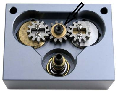
Put a key in one of the cylinders and turn it 180 degrees. Now install the timing gear and shoulder bolt between the cylinders as shown above.
