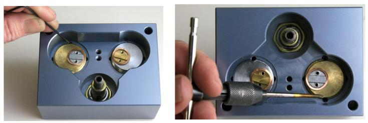
Secure cylinders with two 6-32 set screws. When installing the second set screw it may be necessary to run a 6-32 tap down the side of the cylinder prior to installing.
