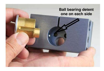
There are two ball bearing detents inside the cylinder clamp. The detents will center the mortise cylinder in the clamp.
