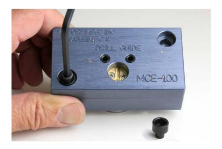
Remove the drill guide from the cylinder clamp. Do not remove the mortise cylinder at this time.
