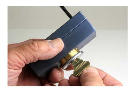
Rotate the key and make sure the cylinder rotates freely on the drill guide. This will insure that everything will be aligned when drilling.
