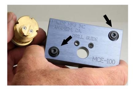
Install the drill guide plate (gray plate) on the cylinder clamp. Do not tighten the mounting screws (see arrows) at this time. The drive cam must be installed at this time, it is used to center the mounting holes.
