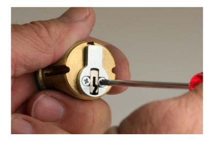
Remove the factory cam.
