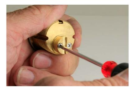
Install the proper cam driver in place of the lock cam.
