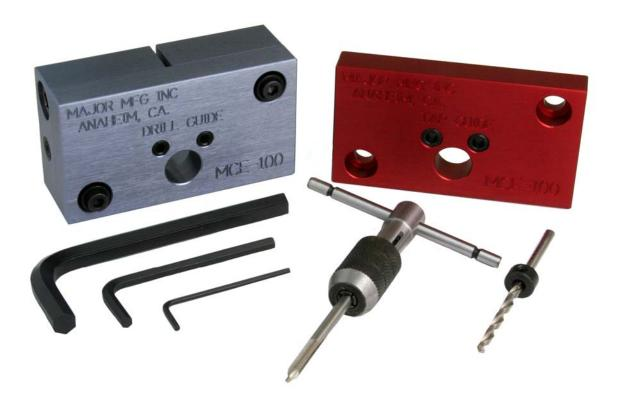
The MCE-100 drill guide is made up of a clamp to securely hold a mortise cylinder when drilling and tapping the required mounting holes. There is also the drill guide plate (gray) and tapping plate (red). Also included is the #29 drill bit with a stop and a 8-32 tap with a handle.
