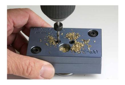
Drill both holes with a #29 drill bit. Adjust the stop on the drill bit so the hole is drilled to a depth of about 3/4" (Adjust the stop so it is 1-1/4" above the tip of the drill bit.) This will allow plenty of room for to tap to the depth needed without bottoming out.
