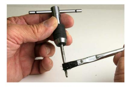
Be sure to lube tap with a cutting oil prior to tapping holes.
