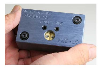
Make sure the mortise cylinder bottoms on the drill guide. There should be no space between the clamp and the drill guide.
