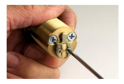
The mortise extension unit Is designed to accept a Kaba Ilco brand cam. The use of other brands may not fit correctly and cause a problem with proper operation.
