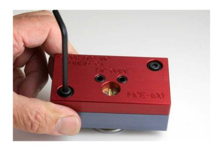
Install the tap guide on the clamp. The cap screws should be loose to allow the guide to float. This will allow the guide to self-align.
