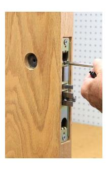
The cylinder hole is large enough to remove the HIT -22 without having to remove the mortise lock from the door. Simply screw the extractor handle into the HIT-22 guide, loosen the mortise cylinder retaining screw and the HIT-22 can be removed.
