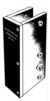
Drill one 1/4" hole through door, enlarge to 3/4" with the use of a hole saw after HIT-110 template has been removed from door.
