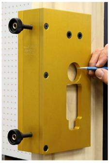
The hole shown at the left is for the rim cylinder. Only route this hole if your panic hardware requires a cylinder. Route to a depth of 1-1/4". Do not attempt to route full depth with one pass. Route in small passes of no more than 1/4" at a time.
