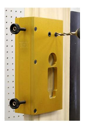
Post holes being drilled on outside of door. Drill size is 3/8" and the depth depends on the length of the post or sex bolt.
