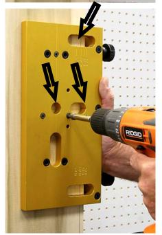
Attach the guide to the door with the supplied #6 dry wall screws. The attaching holes will be on the inside of the door. Use a drill with a clutch system so you don't snap the screws off when they bottom out in the countersink. The screw holes will be covered by the head of the device after it is installed, they will not be visible.
