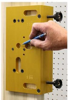
We are now on the inside of the door, this hole is for the rim cylinder tailpiece. Route this through to the hole on the other side.
