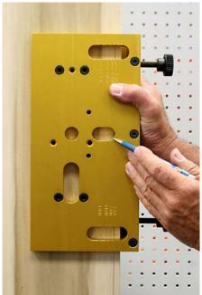
Align the router guide to the proper height using the alignment mark shown in the window.
