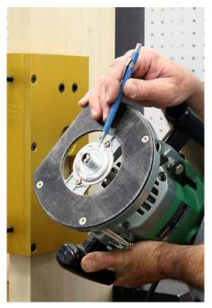
Make sure your router is equipped with the proper sized router guide and bit. This Installation requires a 5/8" outside diameter template guide with a 1/2" diameter up shear router bit. The router bit needs to be adjusted so it is inside the template guide when the router is in the top of the plunge position. ( Part number for our router bit is HIT-45RB8 )
