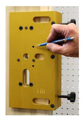
These drill guides are only used if installing the XP99 series device. They are drilled with a 1/8" drill bit and are used to install screws in the panic head.
