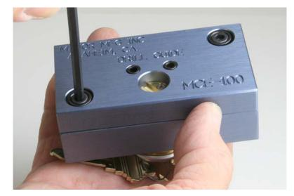
Once the cylinder rotates freely in the drill guide tighten the two cap screws. After the guide has been tightened, check to make sure the cylinder still turns free, if not, readjust. This step is important to insure a good working modification.
