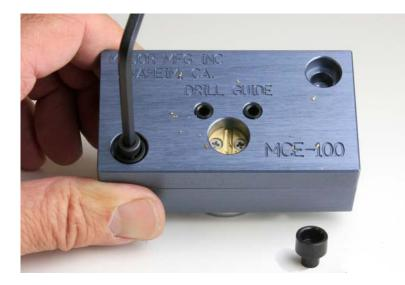
Remove the drill guide from the cylinder clamp. Do not remove the mortise cylinder at this time.
