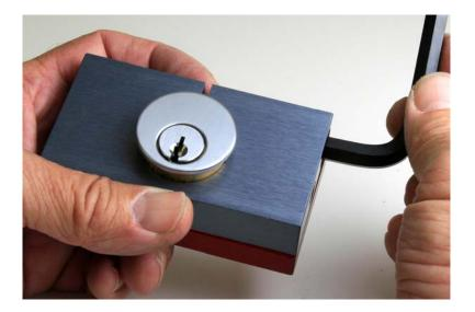
Loosen the cap screw on the cylinder vise and remove the mortise cylinder.
