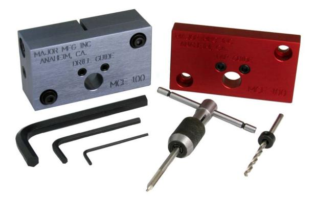
The MCE-100 drill guide is made up of a clamp to securely hold a mortise cylinder when drilling and tapping the required mounting holes. There is also the drill guide plate (gray) and tapping plate (red). Also included is the #29 drill bit with a stop and a 8-32 tap with a handle.
