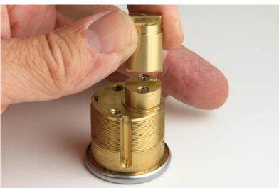
Set the plug extender on the cam driver.
