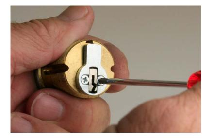
Remove the factory cam.
