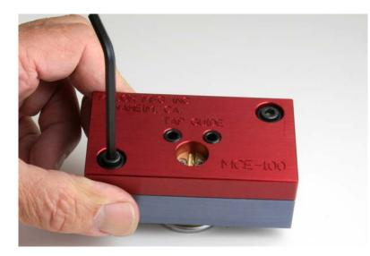
Install the tap guide on the clamp. The cap screws should be loose to allow the guide to float. This will allow the guide to self-align.
