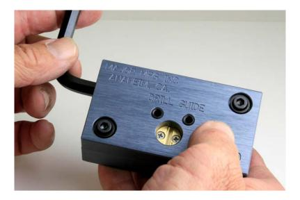
Tighten the mortise cylinder in the clamp unit.
