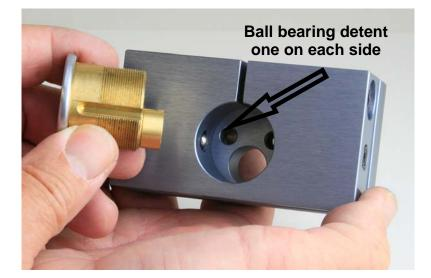
There are two ball bearing detents inside the cylinder clamp. The detents will center the mortise cylinder in the clamp.
