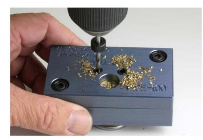
Drill both holes with a #29 drill bit. Adjust the stop on the drill bit so the hole is drilled to a depth of about 3/4" ( Adjust the stop so it is 1-1/4" above the tip of the drill bit.) This will allow plenty of room for to tap to the depth needed without bottoming out.
