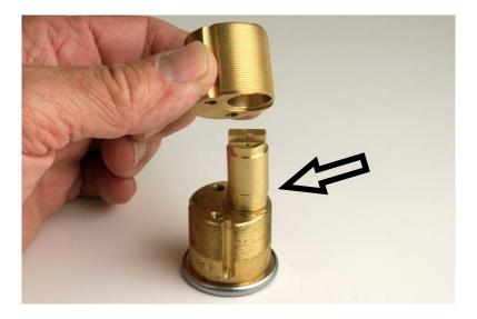
The plug extension will just set on the cam driver, it is captured by the housing when installed. Put the housing over the extension and make sure the plug extension mates with the cylinder plug, see arrow.
