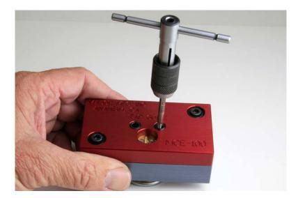
With the use of the red tap guide tap the first hole. Back out the tap frequently to clear chips from work.
