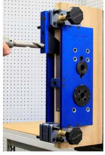
Drill this hole to a depth of 1-1/2". When drilling this hole, back the bit out a few times to clear out the chips.
