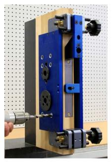
Start by drilling all of the holes located by the silver color drill bushings. Drill size is 7/16", drill half way from both sides of the door. There are a total of six holes to drill.
