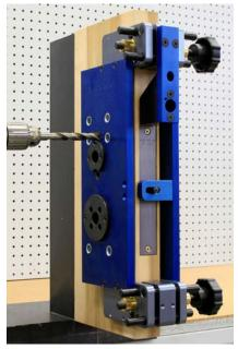
If installing a lock with a door position switch, drill a 1/2" diameter hole on the inside only. Drill a little past center, this hole will meet up with the angled hole drilled in the next step.
