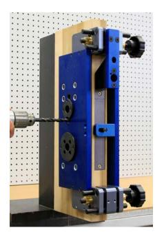
If your AD Mortise Lock is equipped with a dead bolt function, drill the DB hole at this time. NOTE: The factory template calls for a 5/8" hole, a 3/8" hole will work perfectly. Drill to mortise pocket on inside of door only.
