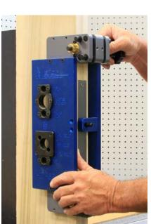
Remove the HIT-66 clamp, template and alignment plate from door.
