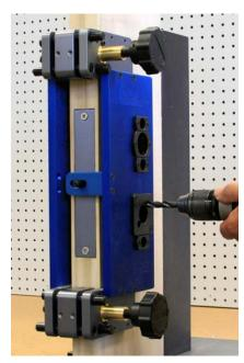
With a 3/8" twist drill, drill the through bolt holes next. Drill to the mortise pocket from both sides of the door.
