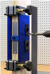
With the 5/8" bit still in the drill, drill the hole required for the thumb turn if required. This hole is drilled only on the inside and not through to the outside of the door.
