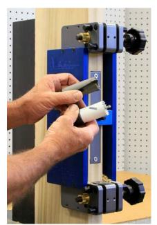
Use a 1-1/4" hole saw and drill for the mortise cylinder. A standard hole saw will work on wood or steel door. Our HIT-48-114 carbide tip hole saw can also be used on wood doors only.
