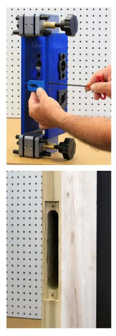
With both clamps opened equally, install both inside and outside templates to the HIT-66 clamp as shown. Do not tighten the 10-32 screws at this time. When all screws have been loosely installed, then it is ok to tighten.
