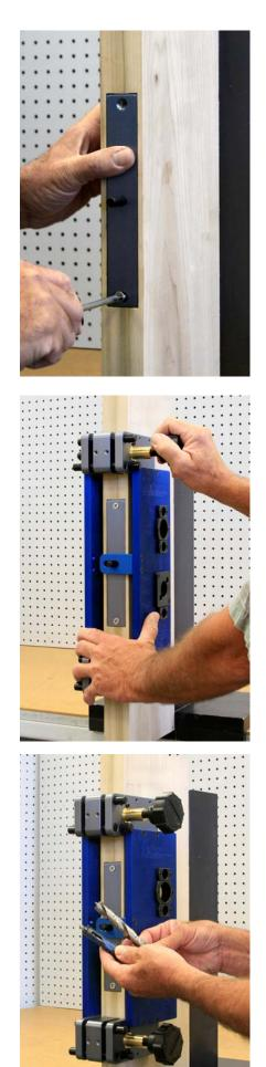
Install the mortise lock positioning plate. The plate will fit into the 1-1/4" x 8" faceplate cut out. There will be a 3/8" diameter pin centered on the plate. There is no top or bottom to worry about.
