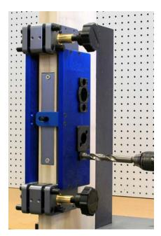
The top and bottom 5/8" diameter holes for the escutcheon trim are being drilled in this step. Be sure to drill only half way from both sides of the template. In the picture we are using a brad point bit, a quality hole saw may also be used on both wood and metal doors.
