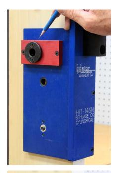
This is the 5/8" hole required for the wire run and inside stud. Be sure to mount this so it is correct for the hand of the door. It can be installed to the HIT-146 fixture on both the right or left hand side. Use a standard twist drill or a brad point bit for wood doors.
