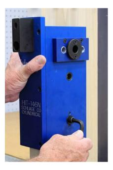
Install both templates to the door, and fasten in place with the supplied socket cap screw. Snug the two templates together with the Allen wrench.
