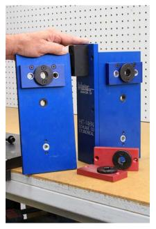
The template set consists of both inside and outside drill guides. All required holes are lined with hardened bushings.
