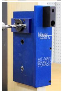
Start by drilling the two silver 7/16" holes on either side of the door. Drill only half way from each side. When drilling pull the drill out to remove chips.
