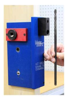
You will need an extra long 3/8" diameter drill bit to drill the angle hole from the door edge to the 1/2" cross bore hole.
