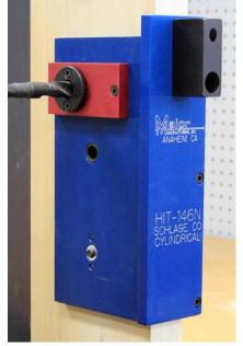
Drill half way from both sides of the door. When drilling pull the drill out several times to help remove chips.
