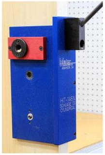
When drilling this angled hole be sure to pull the drill bit completely out of the guide to remove chip build up. Drill 1/2" at a time then clear out chips. This will produce a clean hole and longer drill bit life.
