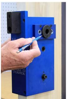
Install the two blue templates to the HIT-146 guide with the use of the supplied 10-32 socket flat head screws. These templates are used to drill the two 7/16" thru-bolts. The center 5/8" drill guide is for steel door installations only. It is for the wire run. Do not drill on a wood door or outside of a steel door. If installing on a steel door, a hole saw may be used.
