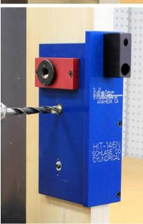
If installing a DPS switch, use a standard 1/2" diameter twist drill on a wood or steel door. A brad point bit may be used on a wood door only. A steel door can be drilled on the inside only. A wood door can be drilled through or just over 1/2 way.
