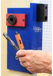
A 5/8" standard twist drill may be used on a wood or steel door as well as a hole saw. A brad point bit may also be used on a wood door only.
