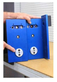
On the inside of the template set are alignment washers. They will drop into the existing cross bore and align the guide to the door.
