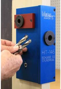
If installing a DPS switch, use a standard 1/2" diameter twist drill on a wood or steel door. A brad point bit may be used on a wood door only.
