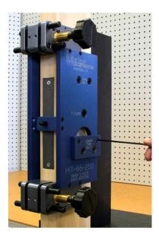
Using the supplied 10-32 x 3/4" flat head screws, install the 1/4" diameter drill guide first. It is easier to drill the smaller hole first as they are located at the very edge of the 2-1/8" hole.
