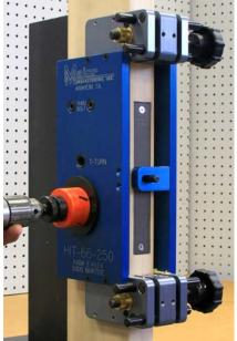
Using a hole saw, drill these holes, use a slow speed on the drill.
