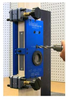
The last hole needed is for the t-turn spindle. Use a 1/2" diameter drill bit and drill both sides of the door.
