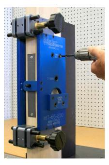
With the 1/4" bit still in the drill, drill the top holes. Again drill half way from both sides of the door.
