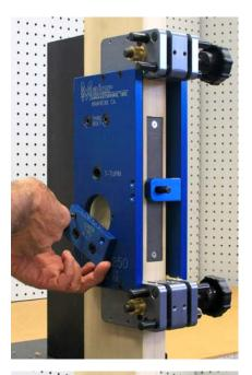
Remove the 1/4" drill guide from both sides of the guide and replace with the 2-1/8" hardened guide.
