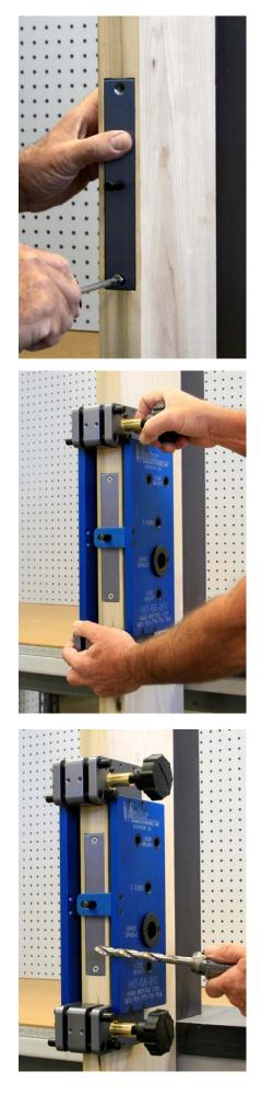
Install the mortise lock positioning plate. The plate will fit into the 1-1/4" x 8" faceplate cut out. There will be a 3/8" diameter pin centered on the plate. There is no top or bottom to worry about.
