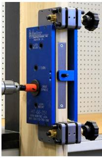
The center 1" diameter guide bushing is for the drive spindle. A hole saw shown at left can be used on both wood or steel doors, dill half way to the mortise pocket from both sides of door.
