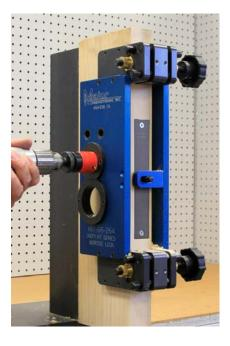
Change to a 1-1/2" hole saw and drill the two 1-1/2" holes to the mortise pocket.
