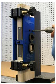
When all holes have been drilled remove the The HIT-66 drill guide from the door.
