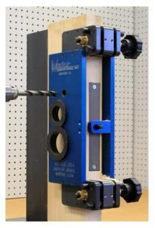
Using a 1/2" twist drill, drill the two upper holes.
