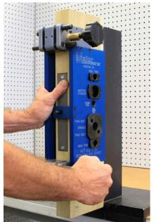
Slide the HIT-66 template with the alignment guide alignment pin and tighten to door. Alternate tightening between the top and bottom clamp. Do not attempt to tighten one clamp all the way at once.
