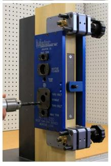
With a 3/8" twist drill, drill the thru bolt holes on both sides of the door. These holes go to the mortise cavity. Drill both top and bottom holes on both sides of the guide, do not try to drill from one side through to the other.
