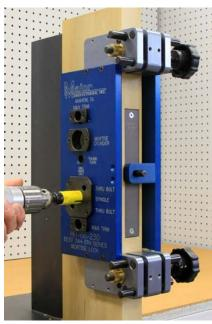
Using a 7/8" hole saw, drill the hole for the lock spindle. It is drilled to the mortise cavity. Drill from both sides of the door.
