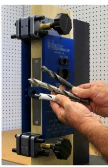
If installing escutcheon trim, the holes can be drilled with a twist drill, brad point bit, or hole saw. If using a brad point bit, it is for use on wood doors only.
