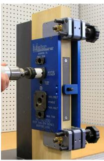
Use a 1-1/4" hole saw to drill the mortise cylinder hole on the outside of the door.
