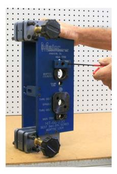
To drill the escutcheon holes for the J trim, remove the hardened drill guides from the M&N trim at the top of the drill guide. Using the same screws, replace with the drill block marked J trim.
