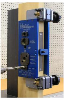
For M & N trim, use a 5/8" bit and drill holes top and bottom using the drill bushings marked M & N. Drill the escutcheon holes half way from both sides of the door.
