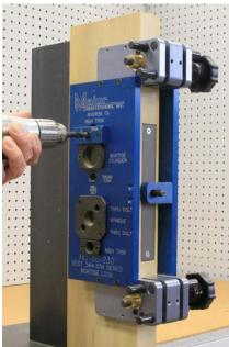
Using a 3/8" twist drill, drill this hole half way from both sides of the door.
