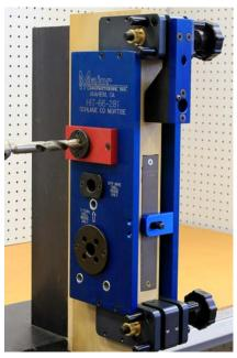
Drill half way from both sides of the door. When drilling pull the drill out several times to help remove chips.
