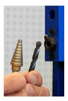
Next drill a 5/16" diameter hole. Drill this hole to 3/4" with the use of a step drill as shown. After the HIT-66 drill guide has been removed from the door. Use care and do not drill hole too big!
