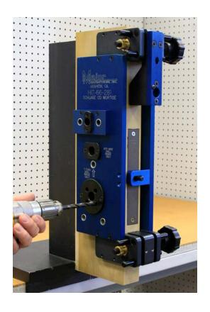
Drill the four 3/8" holes located around the 3/4" spindle hole. Drill to the mortise pocket from both sides of the door.
