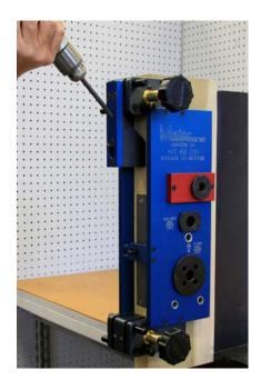
Using a 5/16" diameter long drill bit, drill to the mortise pocket. When drilling a deep hole, pull the bit out when drilling to remove chips.
