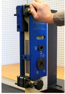
Slide the HIT-66 set up alignment fixture over the alignment pin and tighten to door. Alternate tightening between the top and bottom clamp. Do not attempt to tighten one clamp all the way at once.
