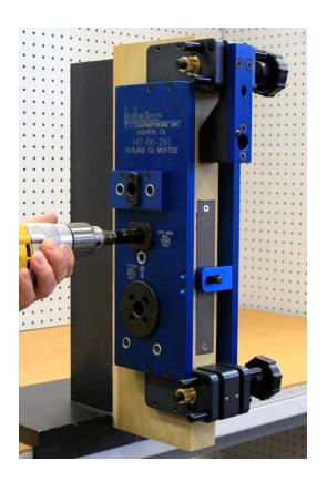
With the 3/4" hole saw still in the drill, drill the 3/4" wire run hole. This hole is drilled on the inside of the door only.
