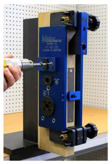
Start by drilling the four holes located in the corner of the template. Drill size is 7/16", drill half way from both sides of the door. Use a twist drill for wood or metal doors.
