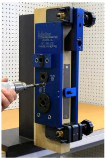
If your CO Mortise Lock is equipped with a dead bolt function, drill the DB hole at this time. NOTE: The factory template calls for a 5/8" hole, a 7/16" hole will work perfectly, and you already have it in your drill. Drill to mortise pocket on inside of door only.
