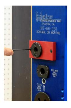
This is the red drill template required 5/8" diameter wire run and inside stud. Be sure to mount this so it is correct for the hand of the door. It can be installed to the fixture on both the right or left hand side. Use a standard twist drill or a brad point bit for wood doors.
