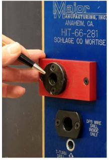
The red template should be mounted on the outside of the door to match the door handing.
