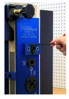
Install the two blue templates to the guide with the use of the supplied 10-32 socket flat head screws. These templates are used to drill the two 7/16" thru-bolts. The center 5/8" drill guide is for steel door installations only. It is for the wire run. Do not drill on a wood door or outside of a steel door. It is used for the inside of a steel door only.
