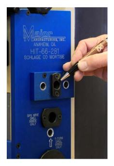
The blue template is on the inside and will be drilled in the center.
