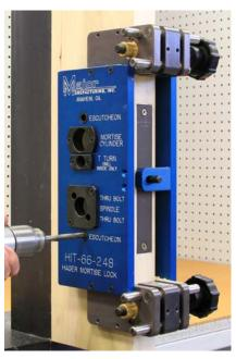
With the 3/8" bit still in the drill, drill the top and bottom escutcheon trim holes. Drill these from both sides of the drill guide.
