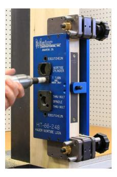
Use a 5/8" diameter hole saw to drill the hole for the thumb turn. This hole is drilled on the inside and drilled to the mortise pocket.
