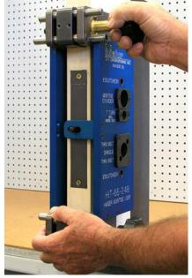
Slide the HIT-66 template guide onto alignment pin and tighten to door. Alternate tightening between the top and bottom clamp. Do not attempt to tighten one clamp all the way at once.
