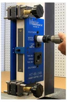
Use a 1-1/4" hole saw to drill the mortise cylinder hole on the outside of the door. Again, back the hole saw out a few times to clear saw dust from the cut.
