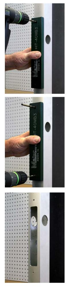
Drop into the cut out. If the lock was correctly installed there should be no top to bottom play. Drill one of the holes as shown.
