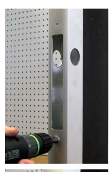
Counter sink both holes so the 10-32 machine screw is flush.
