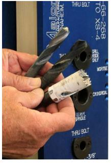
Shown are drill bits that will work with this drill guide. The twist drill will be a good choice for both wood or steel doors, The hole saw will be needed for larger holes. Do not use spade type bits, there is no bearing surface and they will jamb in the drill guides.
