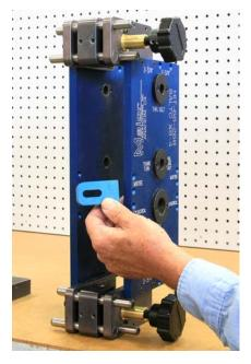
Install the yoke shape alignment guide with 2 10-32 screws as shown. Mount the guide in the holes marked mortise, it can be mounted on either side of the guide.
