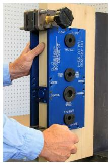
Alternate tightening between the top and bottom clamp. Do not attempt to tighten one clamp all the way at once.
