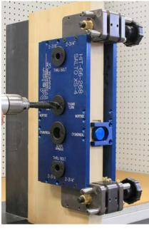
Switch to a 5/8" bit and drill the hole for the thumb turn if needed for the function of lock being installed. On a cylindrical this hole goes through the door. Drill half way from both sides of the door.
