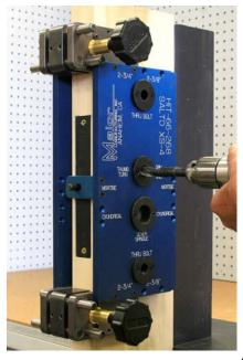
If the lock function you are installing requires a t-turn, drill a 5/8" hole to the mortise pocket on the inside only.
