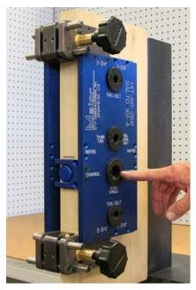
Since we are installing a cylindrical lock and the hole for the lever spindle is centered over the existing cross borehole, it is not needed.
