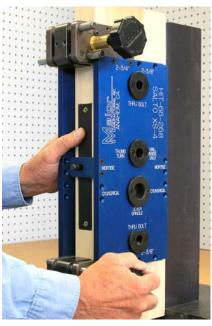
Slide the HIT-66 alignment fixture over the alignment pin and tighten to door.
