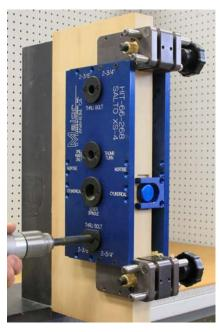
Using a 9/16" drill bit drill the thru bolt holes, drill half way from both sides of the door. Drill both top and bottom
