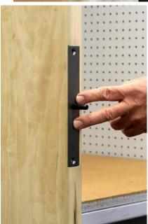
Install the mortise lock positioning plate.
