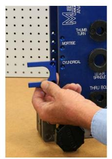
Install the "U" shape alignment guide with 2 10-32 screws as shown. Mount the guide in the holes marked cylindrical, it can be mounted on either side of the guide.
