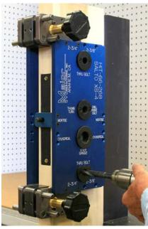
Using a 9/16" drill bit, drill the holes needed for the thru bolts. Drill the top and bottom holes half way from both sides of the door.
