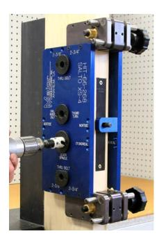
Drill the 1" hole for the lever spindle half way from both sides of the door, this hole will go to the mortise pocket.
