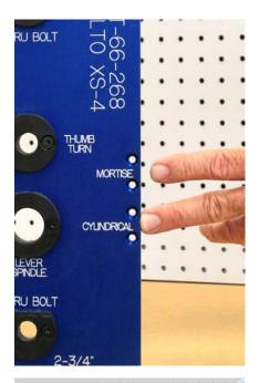
The HIT-66-268 drill guide for Salto XS-4 locks can be set up for use for both cylindrical and mortise locks. It is also adjustable for both 2-3/8" and 2-3/4" backsets.
