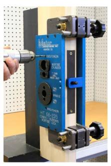
The drill bushings on this template are 6-3/4" center to center. Make sure this matches the escutcheon trim being installed. The drill bushing diameter is 3/16". This can be drilled out if a larger hole is needed. Drill half way from both sides of the door.
