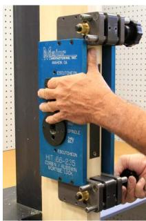
If installing rose trim, the installation is now complete. Remove the clamp and template from the door and install the mortise lock per the manufacturers instructions.
