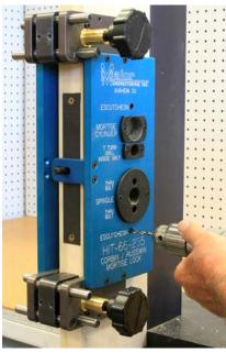
If the escutcheon trim is mounted with screws and not thru bolted, mark the locations after the drill guide has been removed from the door and drill for wood screws or drill and tap if on a steel door.
