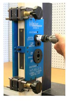
Use a 1-1/4" hole saw and drill for the mortise cylinder. A standard hole saw will work on wood or steel door. This hole is to be drilled only on the side of the door that will have the cylinder installed.
