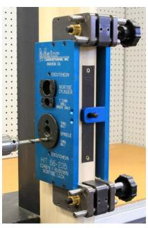
Drill both sides of the door above and below the spindle hole
