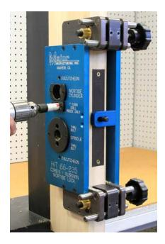
If installing a thumb turn, use a 5/8" hole saw and drill only on the side of the door that requires the turn. This hole will go to the mortise pocket.
