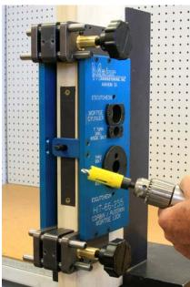
Drill the spindle hole using a 7/8" hole saw. Use a slow speed and back the hole saw out of the cut when drilling to remove chips.
