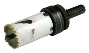
All hole saws are not created equal. A cheap hole saw from a home improvement center or one that has been dropped can be out of round and will not fit the drill bushings in our templates.
