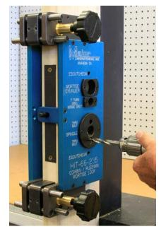
Using a 3/8" drill bit drill the top and bottom thru bolt holes, these holes go only to the mortise pocket.
