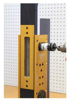
Once the faceplate has been cut out it is time to start drilling the function holes. Starting at the top, drill the inside and outside holes with a 1-1/4" hole saw. If retrofitting, drill these holes to clean up any misalignment.
