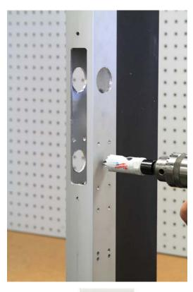
One last hole to enlarge is on the interior of the door. Change to a 7/8" hole saw and drill the pilot hole located under the two horizontal holes as shown.
