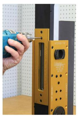
Don't forget to drill the holes for mounting brackets. The holes in the template are spaced to fit our LMB-03, LMB-033 or LMB-034. We prefer the bracket to mounting bridges for this installation.
