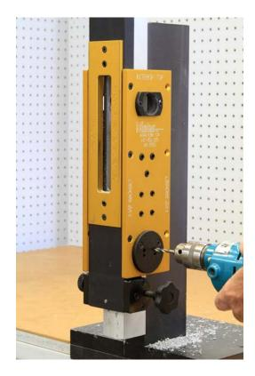
With the 13/64" drill bit still in the drill, drill the two top holes on the large drill guide at the bottom of the template
