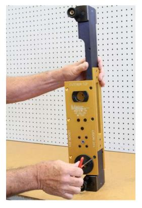
The templates are marked exterior top and interior top make sure they are attached correctly to the clamp. There are mounting holes on both the right and left hand side. One is for 1-1/8" and the other 1-1/2" backset. The screws go through the backset that is required.
