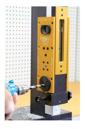
There is one last hole to drill. With a 1/2" twist drill, drill the bottom hole in the large drill bushing. This is on the exterior template.
