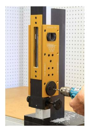
Change to a 3/16" and drill the remaining 6 holes on the inside template. Four are on the template and two are on the large drill guide.
