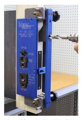
With the brad point bit touching the door, mark 1-1/2" on the bit with a felt pen or use a piece of tape. This will be your stop mark.
