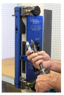
There are three 5/8" holes on each side of the template. One is for escutcheon trim and are drilled thru. One is for a T-turn and drilled INSIDE ONLY. The last 5/8" hole is for a wire run from inside to outside of the door. A hole saw can be used or a brad point bit can be used on a wood door only.
