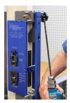
Using a 5/16" diameter long drill bit, drill to the DPS hole drilled in the step above. When drilling a deep hole, pull the bit out when drilling to remove chips.
