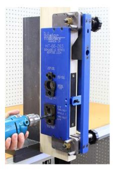
Start by drilling all of the 3/8" thru bolt holes. Drill half way from both sides of the door. There are a total of four holes to drill on both sides of the door. Two around the lock spindle and two on the upper part of the template.
