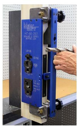
If the lock being installed is a deadbolt function, two more holes will be needed. A 3/4" hole to a depth of 1-1/2" and a 40 degree hole to the 5/8" wire hole located between the two top thru bolts. On a wood door, use a 3/4" brad point bit. On a steel door see special directions on page 8.
