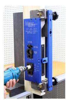
Using a good quality hole saw, drill the spindle hole using the drill bushing shown in the picture. The hole saw size is 1" and is drilled to the mortise pocket on both sides of the door. Use a slow speed when drilling.
