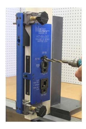
Upper and lower trim holes being drilled with a 5/8" drill bit. Be sure to drill half way from both sides of the door.
