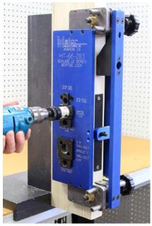
With a 1-1/4" hole saw, drill the mortise cylinder hole. This hole is drilled on the **OUTSIDE ONLY** and to the mortise pocket
