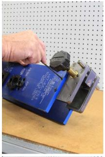
With both clamps opened equally, install both inside and outside templates to the HIT-66 clamp as shown. Do not tighten the 10-32 screws at this time. Tighten only after the drill guide for the deadbolt function has been installed on the front of the drill guide.
