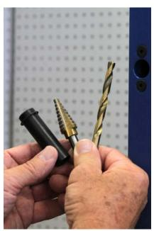
If installing a deadbolt function on a steel door, use the supplied 3/4" to 5/16" hardened adapter (shown on left) Slide this into the 3/4" drill guide on the front of the door and drill with a 5/16" twist drill. After all holes are completed and the HIT-66 is removed from the door, enlarge the 5/16" hole to 3/4" with the use of a step drill. Do not attempt to drill this hole with a hole saw. The finished hole will be too large.
