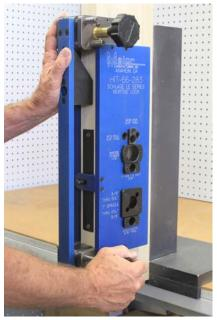
Slide the HIT-66 set up alignment fixture over the alignment pin and tighten to door. Alternate tightening between the top and bottom clamp. Do not attempt to tighten one clamp all the way at once.
