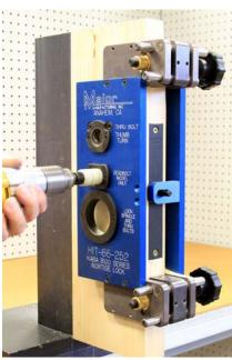
The next hole down is marked Dead Bolt Hole Only. It is a 1" diameter hole and can be drilled thru the door using a hole saw, Drill half way from both sides of the door.
