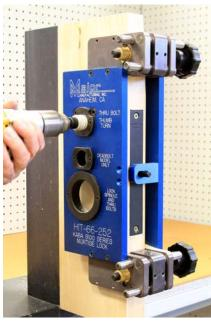
The next hole down is marked thumb turn. It is a 1" diameter hole and can be drilled thru the door using a hole saw, Drill half way from both sides of the door.
