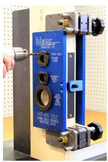
There are two drill guides that are for the thru bolt mounting holes. They are 1/4" diameter. Drill both holes half way from both sides of the door.
